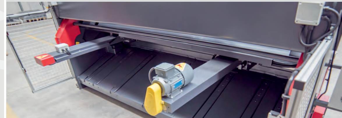
Motorized Back Gauge has \pm 0,1\text{mm} Accuracy
