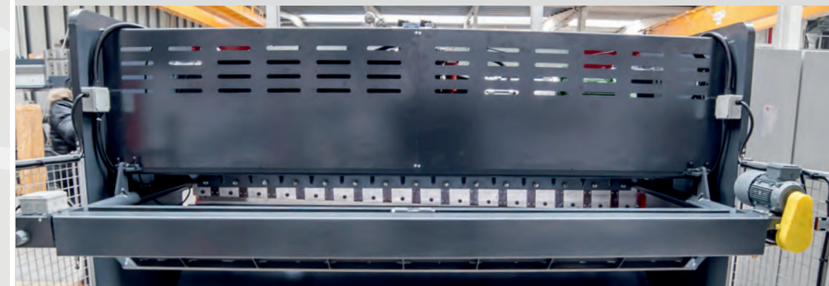
Motorized Back Gauge has \pm 0,1 mm Accuracy
